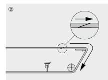
Before fitting the belt on the conveyor, ensure that the conveyor is in perfect operating condition, taking any necessary steps. Clean drums, support rollers and skid plate, removing any residues. Prepare the conveyor for the insertion of the conveyor belt.
