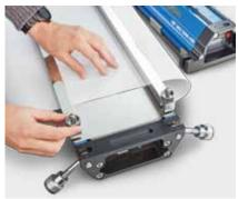
As specified in the Forbo Siegling splicing instructions for different materials, temperature, dwell time and pressure are easy to set. Instructions on the display take the user systematically through the menu. The actual splicing process is carried out automatically.
